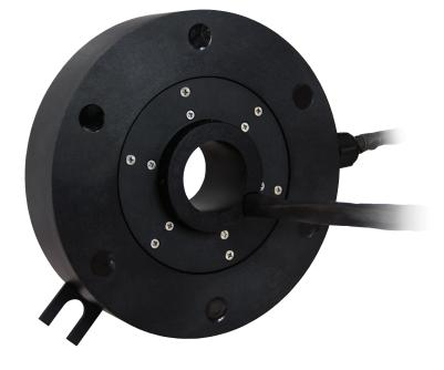
The flat F Series Slip Rings have a special design, that means these rotary joints have a height of only 45 mm ensuring up to 17 signal circuits and 3 power circuits up to 15 A.
